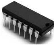
Can also be called a PDIP (plastic dual in-line package)
